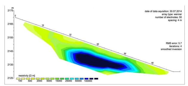
*Figure 3.4.2 Example of a longitudinal ERT profile on Upper Pietricelele rock glacier (after Onaca et al., 2015).*
