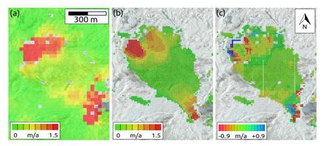
Figure 3.2.1.1: Distelhorn rock glacier (Mattertal, Switzerland). (a) Horizontal velocity map from TerraSAR-X offset tracking between 11.09.2014 and 06.09.2016; (b) Horizontal velocity map from matching of aerial optical images with a spatial resolution of 0.15 m acquired on 03.09.2014 and 21.09.2017; (c) Difference map between aerial photo matching and TerraSAR-X offset tracking velocities (Strozzi et al., 2020).
