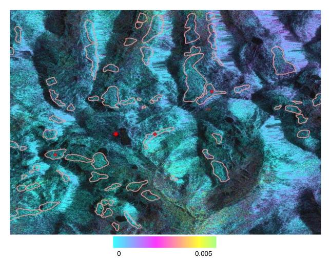
Figure 3.4.13 Measurement noise standard deviation of Sentinel-1 data for selected rock glaciers. Red points indicate rock glacier locations with known dynamics and the red star indicates the location of both GPS and InSAR references.
