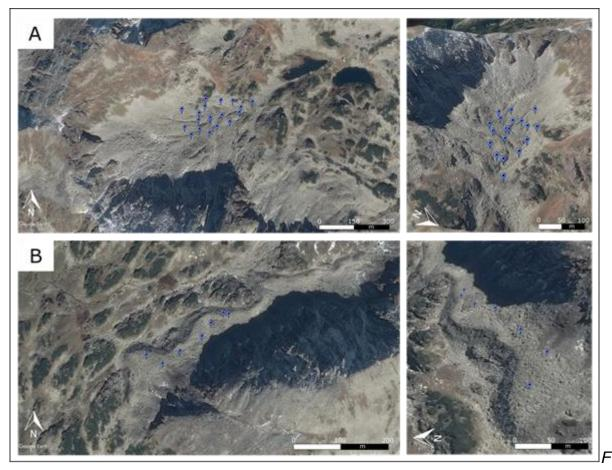
Figure 3.4.1 The distribution of GNSS measurement points (2019 survey) on the Judele (A) and Peleaga (B) rock glaciers (source of the background images: Google Earth, 16.11.2014, 2020 CNES/Airbus).
