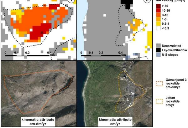
Figure 2.3.2.2: Detailed maps over two high-risk rockslides of Troms study area: 1) Gámánjuuni 3 and 2) Jettan. Both landforms are continuously monitored. In-situ measurements from the Norwegian Water Resources and Energy directorate (NVE) and the Geological Survey of Norway (NGU) show velocity ranges in the similar order of magnitude as the assigned kinematic attribute, based on the InSAR moving areas (MA).
