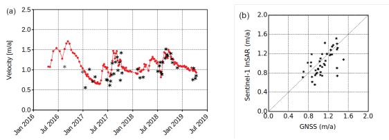
Figure 3.1.3.1: Three-dimensional (3D) GNSS velocities computed with the average daily positions corresponding to the acquisition dates of the Sentinel-1 acquisitions (red diamonds) and velocity along the maximum slope direction from Sentinel-1 InSAR (grey 12 day time interval, black 6 day time interval) at GNSS station BdB2 over Becs-de-Besson rock glacier (Val de Réchy, Switzerland); (b) Scatter plot of GNSS and Sentinel-1 InSAR velocities at 41 measurements points (Strozzi et al., 2020).
