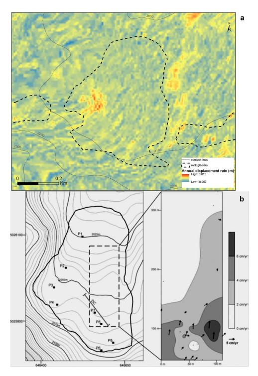
*Figure 3.4.5* Annual displacement rates based on InSAR analysis (Sentinel-1) (a) and geodetic surveys between 2008 and 2009 (b) (after Vespremeanu-Stroe et al., 2012) at Pietrele 1 rock glacier.
