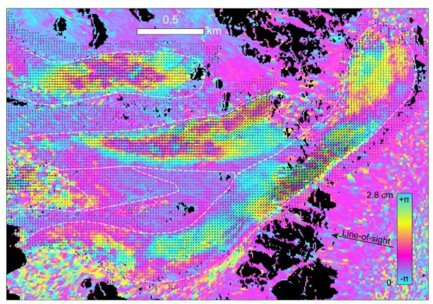
Figure 2.3.6.1: Ordzhonikidze rock glacier, Tien Shan. Section of a interferogram between Sentinel-1 radar data of 24 Aug and 5 Sep 2018 (12 days) with vectors superimposed from image matching between 2016 and 2018 high resolution satellite images. The white dashed lines are the inventory outline polygons from motion and process-type classes. Photogrammetric velocities are up to 4 m/yr. Similar comparisons for the other rock glaciers are displayed in the Supplement of Kääb et al. (2021).
