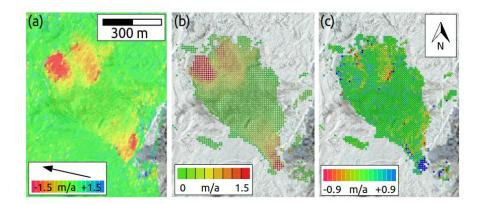
Figure 3.1.3.2: Distelhorn rock glacier (Mattertal, Switzerland). (a) Sentinel-1 InSAR lineof-sight velocity map from 02.08.2018 to 08.08.2018; (b) Horizontal velocity map from matching of aerial optical images with a spatial resolution of 0.15 m acquired on 03.09.2014 and 21.09.2017; (c) Difference map between aerial photo matching and Sentinel-1 InSAR LOS velocities (Reference Strozzi et al., 2020).
