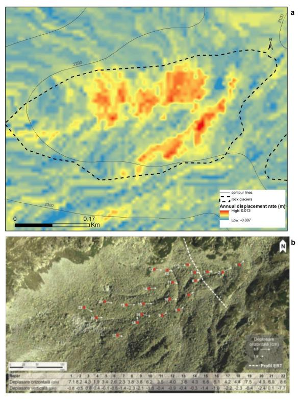
Figure 3.4.6 Annual displacement rates based on InSAR analysis (Sentinel-1) (a) and geodetic surveys between 2012 and 2014 (b) (after Popescu, 2015) at the Judele rock glacier. Horizontal and vertical displacement rates are displayed in the inset table.
