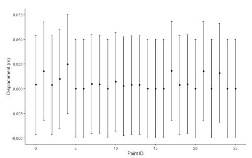
*Figure 3.4.4 Displacement measurements over the Judele rock glacier (A) and 8 points over Berbecilor (B) rock glacier (see Figure 3.4.5) using a differential GPS and instrumental error.*
