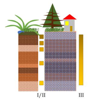
**Figure 4.7:** Permafrost\_cci metadata collection planned on stratigraphy, organic layer, ground ice content, dominating lithology and texture and on the buffer layer (vegetation composition, infrastructure, ...) will be provided at the best quality available and including a quality index (cf. Tables 4.6 - 4.9).
