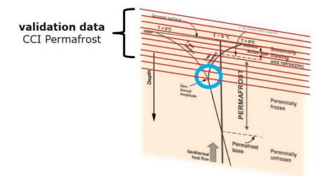
*Figure 4.3:* Concept of Zero Annual Amplitude (ZAA) depth (blue circle) and Permafrost\_cci depth stratification.
