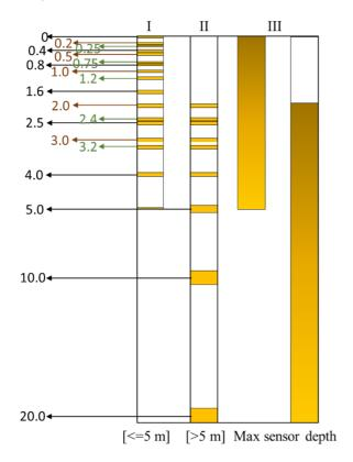
**Figure 4.4:** Discrete depths are provided small-scaled in shallower depths and larger scaled in deeper depths. In deep boreholes (Group II, >5 m depth), <1.5-2 m measurements were discarded due to their inaccuracy due to large borehole diameter and air or artificial infillings. In Group III, temperature data are interpolated for shallow and deep temperature profiles down to the maximum sensor depth. Also here, the upper 1.5-2 m temperature measurements of deep boreholes are discarded.
