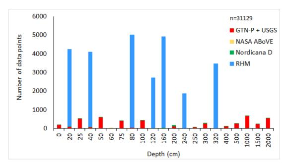
*Figure 4.2:* Number of Ground Temperature (GT) measurements at a given depth (in centimeter, y-axis) which can be used for validation in Permafrost\_cci. Values include measurements over all years from 1980-2022 with n being the overall amount of available GT data per depth.
