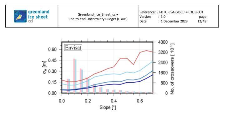
Figure 2.1: Crossover statistics of Envisat over Antarctica from Schröder et al. (2019). Standard deviation as a function of slope. The curves represent different retrackers employed to the data and the vertical bars indicate number of crossovers.
