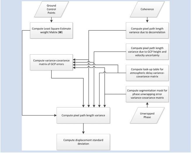
Figure 3.1: Error prediction framework for interferometric displacement measurement.
