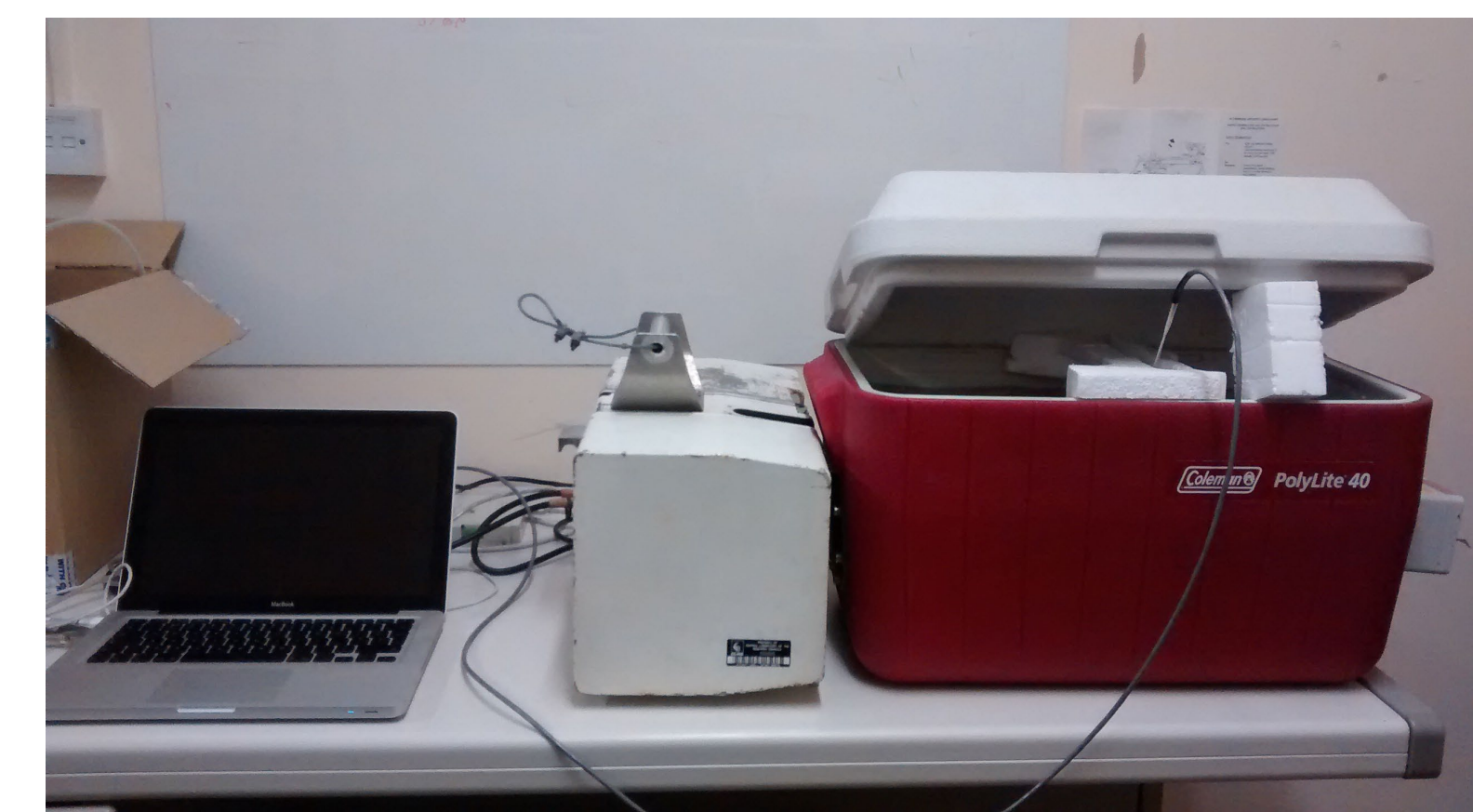
Figure 3: Calibration setup of SISTeR (middle) against the CASOTS blackbody source (right)
