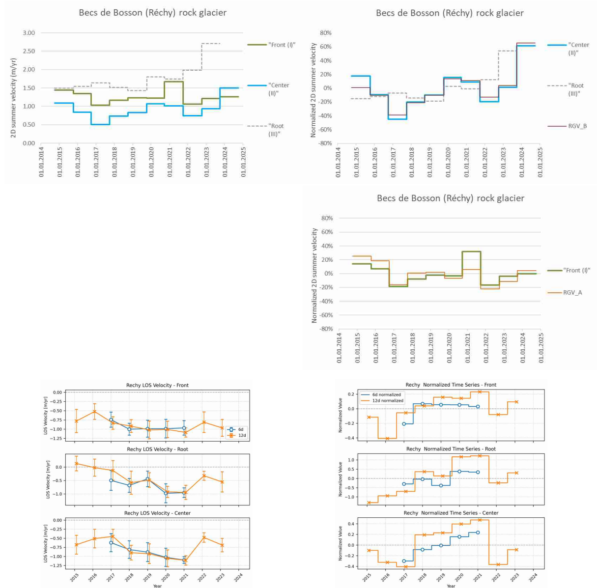
Figure 16. Comparison between available GNSS-RGV data (upper graphs) and Permafrost_cci InSAR-RGV (lower graphs) on Réchy rock glacier. Left: m/yr velocity time series. Right: Relative velocity changes.
