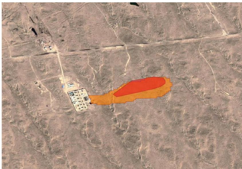
Figure 7.1.2-4: Kayrros (orange) and UPV (red) masks delineated for 20230623 Sentinel-2 plume in TKM1.
