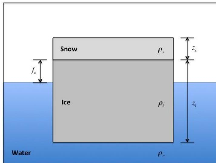
Figure 5-24: Computation of sea ice thickness
