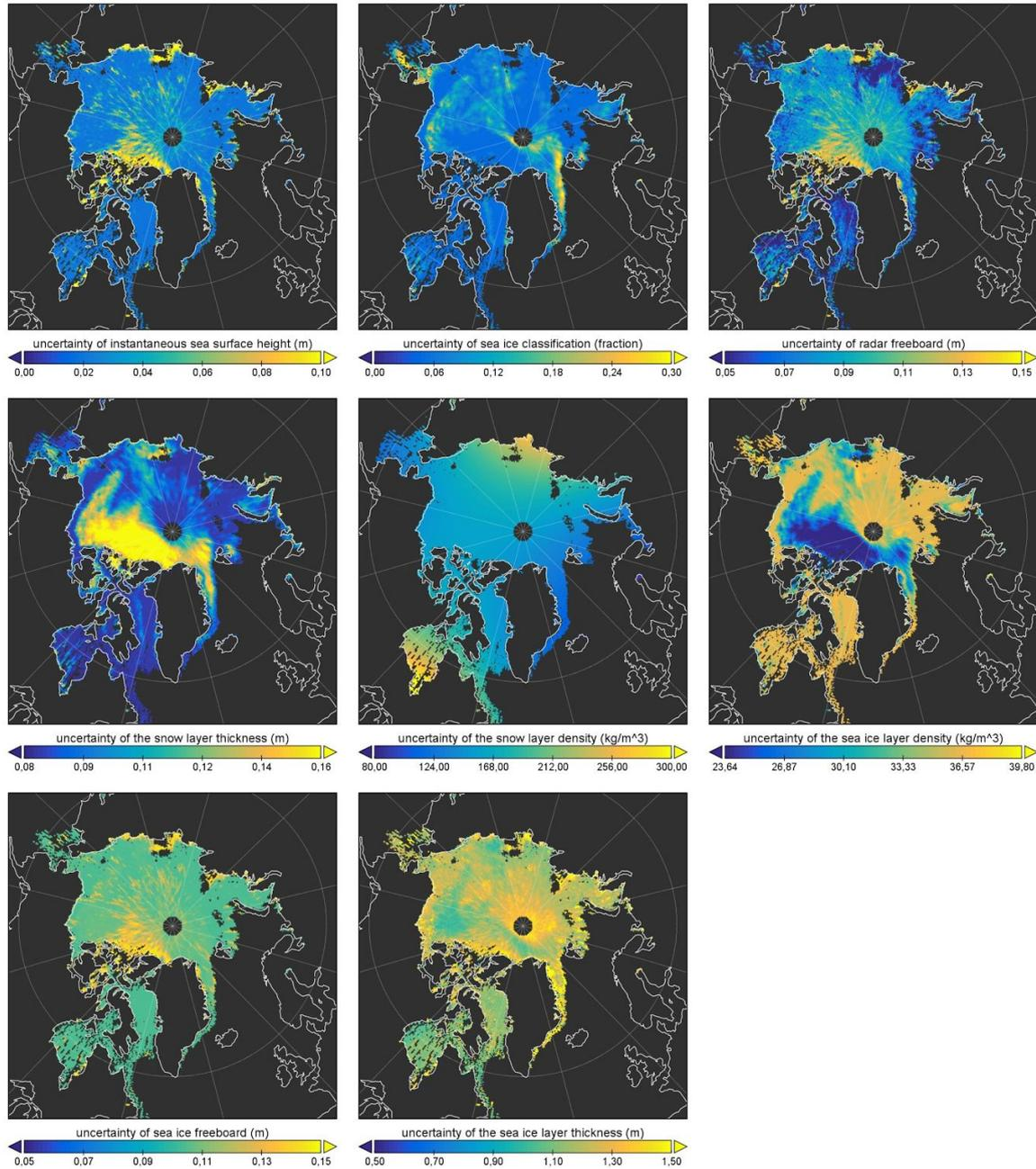
**Figure 6-1: Gridded uncertainties (Example CryoSat-2 March 2015 Arctic data)**
