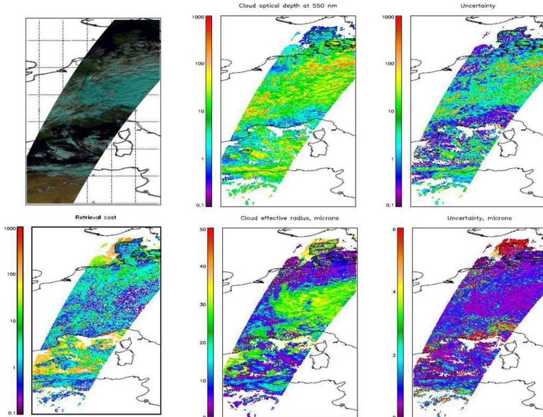
**Figure 2: Example of cloud retrieval over Europe. Top from left to right: false colour image based on instrument swath (blue colour is indicative of ice cloud), cloud optical depth and error on the cloud optical depth. Bottom from left to right: retrieval cost, cloud effective radius and error on the effective radius.**
