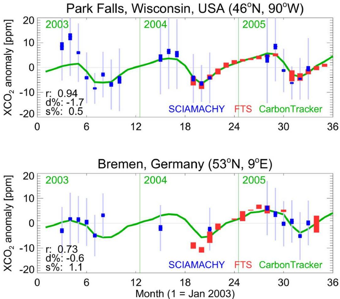
**Figure 4: Comparison of anomalies of column-averaged dry air mole fraction of CO<sub>2</sub> derived from satellite (IUP SCIAMACHY WFMDv1.0 XCO<sub>2</sub> data product), ground-based remote sensing (TCCON FTS) and model-based analysis (NOAA CarbonTracker) for Park Falls, Wisconsin, USA (top) and Bremen, Germany (bottom). The panels also include error bars where available (Schneising et al., 2008).**
