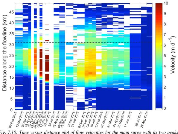
*Fig. 7.10: Time versus distance plot of flow velocities for the main surge with its two peaks. Maximum values reached 14 m per day in May 2015.*
