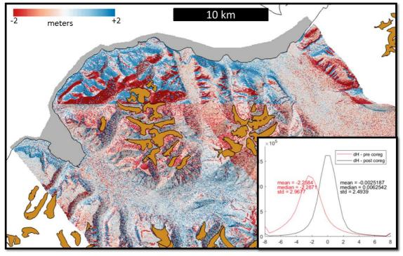
Figure 6.4: Stable terrain elevation differences between the TanDEM-X IDEM product and a national DEM derived from vertical aerial photographs. A distinct linear feature running east-west shows a merging artefact between two adjacent IDEM tiles. The inset shows the histograms of stable terrain differences before and after uniform co-registration between the DEMs.
