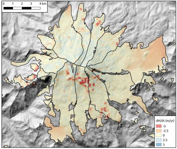
Figure 6.5: Elevation changes over Mt. Elbrus (Caucasus) as derived from ASTER scenes acquired over the 2014 to 2017 period and the SRTM C band DEM.
