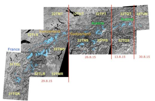
*Fig. 4.3: Glacier outlines (light blue) on top of the Sentinel 2 tiles (band 8 in the near infrared) used for glacier mapping in 2015. Some additional scenes are listed in Table 4.3.*
