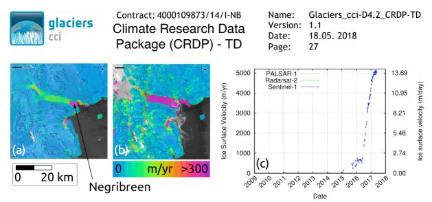
Figure 7.8: Ice surface velocity maps for Negribreen on Spitsbergen (Svalbard) from Sentinel-1 data of the time periods 01/10/2015 to 13/10/2015 (a) and 31/10/2016 to 12/11/2016 (b) and time-series of velocity close to the front from 2011 to 2017 (c). The arrow points to the location used for the time series.
