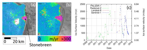
*Figure 7.9: Ice surface velocity maps for Stonebreen on Edgeøya (Svalbard) from Sentinel-1 data of the time periods 21/01/2015 to 02/02/2015 (a) and 27/02/2017 to 11/03/2017 (b) and time-series of velocity close to the front from 2009 to 2017 (c).*
