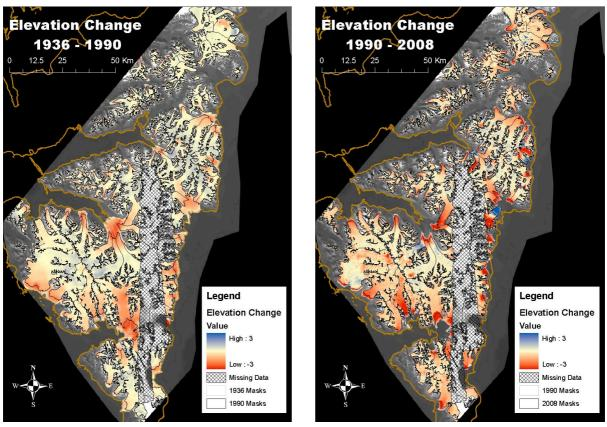
Figure 6.3: Elevation changes from two epochs spanning the past 80 years. The first epoch (left) compares the oldest national topographic maps from Svalbard in 1936 to a DEM derived from vertical aerial photographs in 1990. Right: The second epoch (1990-2008) compares the DEM to a satellite DEM derived from SPOT5 during the IPY-Spirit mission (Korona et al. 2009).
