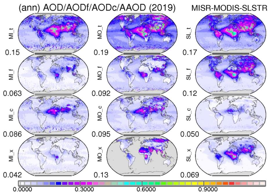
**Figure 3.1** Comparisons of retrieval associated aerosol data between established NASA retrievals by MISR (column1) and MODIS (column2) and ESA's SLSTR. For the year 2019 annual average maps are presented for the total AOD (row 1), the AOD split into fine-mode (row2) and coarse-mode (row 3) and for the total AAOD (here multiplied by 10 to fit the common scale).
