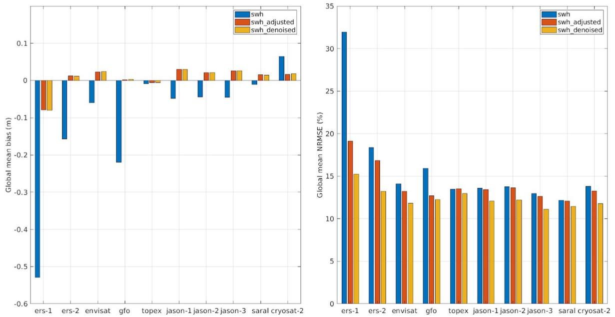
Figure 9. Bias (left) and NRMSE (right) computed from the comparisons between altimeter and wave model hindcast.
