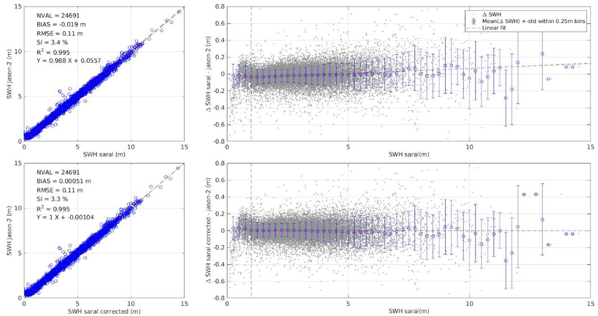
Figure 3. (Left) Scatter diagrams of Jason-2 swH against Saral swH before (top) and after (bottom) calibration. (Right) Residual of Saral swH – Jason-2 swH as a function of Saral swH before (top) and after (bottom) calibration. The red dashed line is a linear fit through the data.
