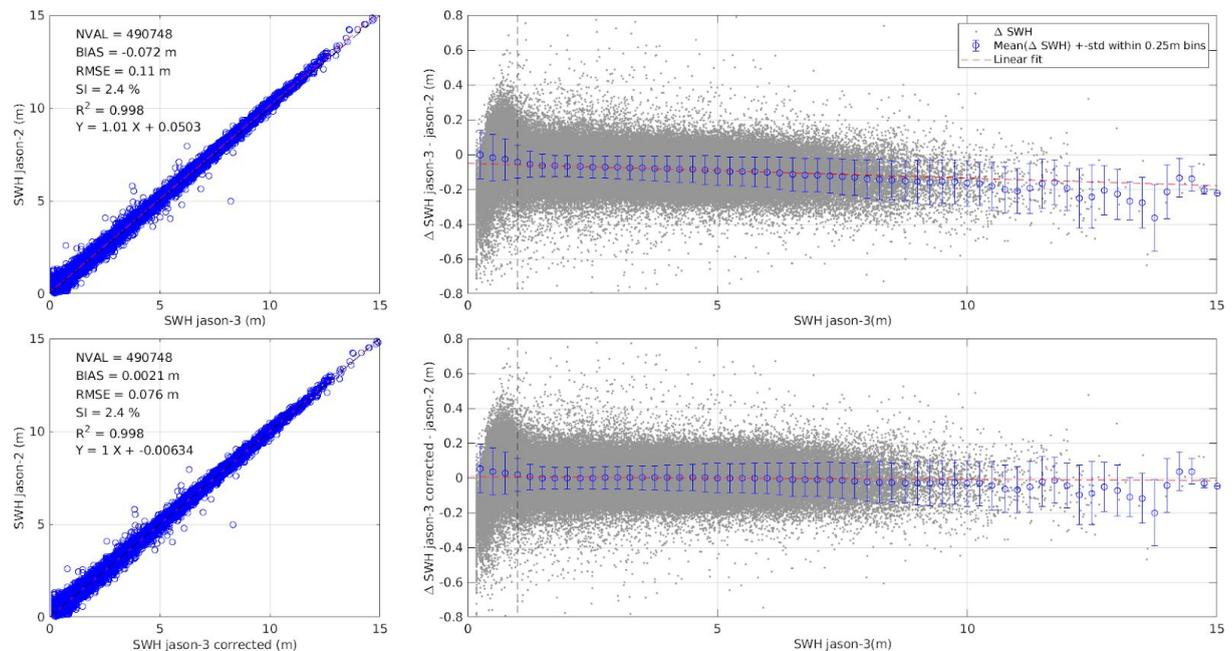
Figure 4. (Left) Scatter diagrams of Jason-2 swH against Jason-3 swH before (top) and after (bottom) calibration. (Right) Residual of Jason-3 swH – Jason-2 swH as a function of Jason-3 swH before (top) and after (bottom) calibration. The red dashed line is a linear fit through the data.
