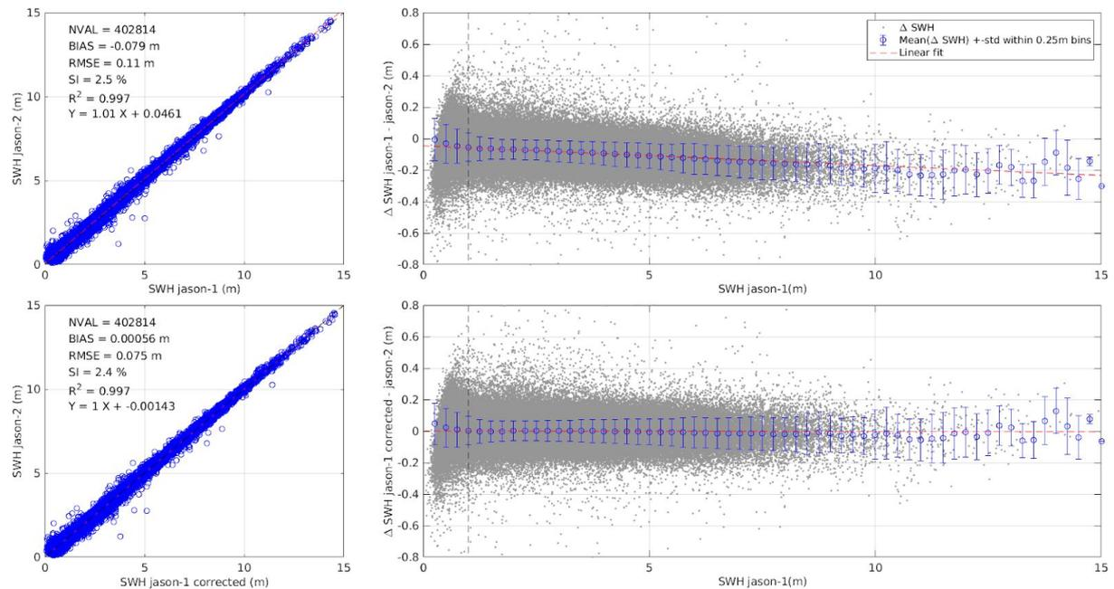
Figure 2. (Left) Scatter diagrams of Jason-2 swh against Jason-1 swh before (top) and after (bottom) calibration. (Right) Residual of Jason-1 swh – Jason-2 swh as a function of Jason-1 swh before (top) and after (bottom) calibration. The red dashed line is a linear fit through the data.
