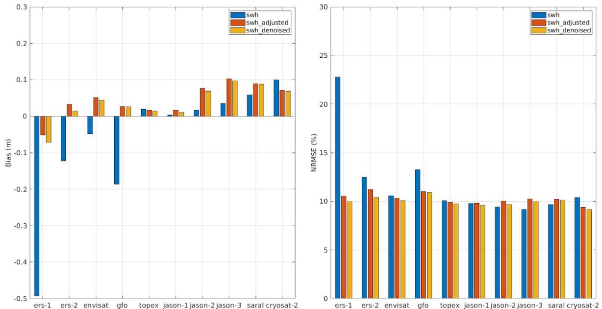
Figure 8. Bias (left) and NRMSE (right) computed from the comparisons between altimeter and in-situ buoy data.
