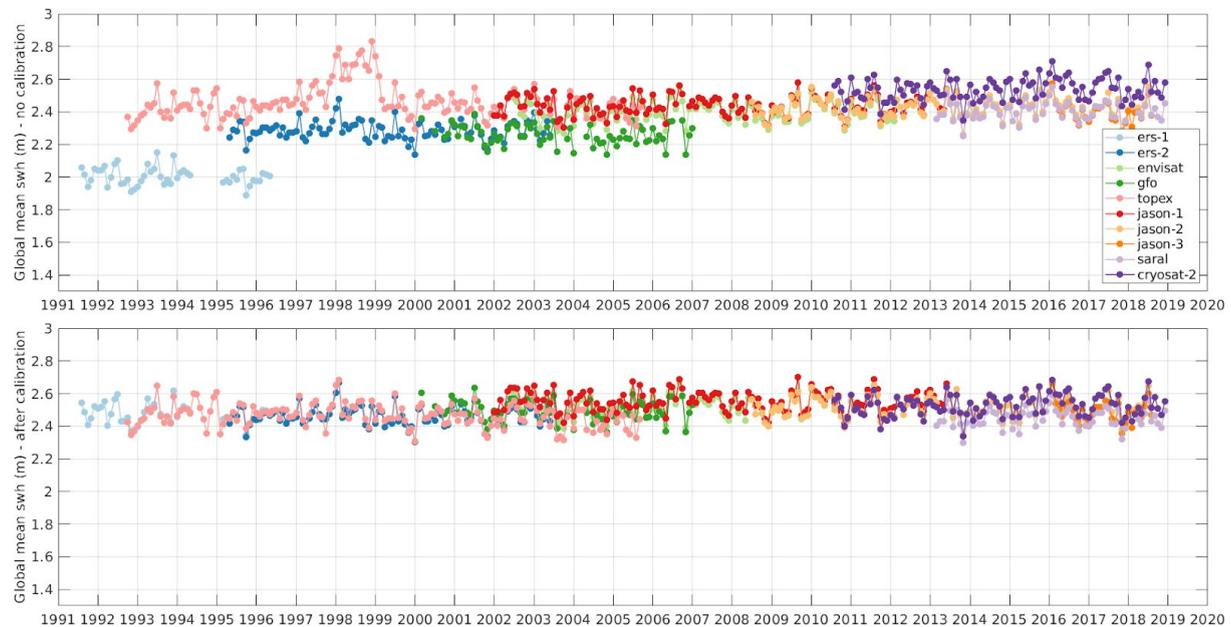
Figure 6. Monthly global mean swh over the period 1992-2018 before (top panel) and after (bottom panel) calibration is applied.
