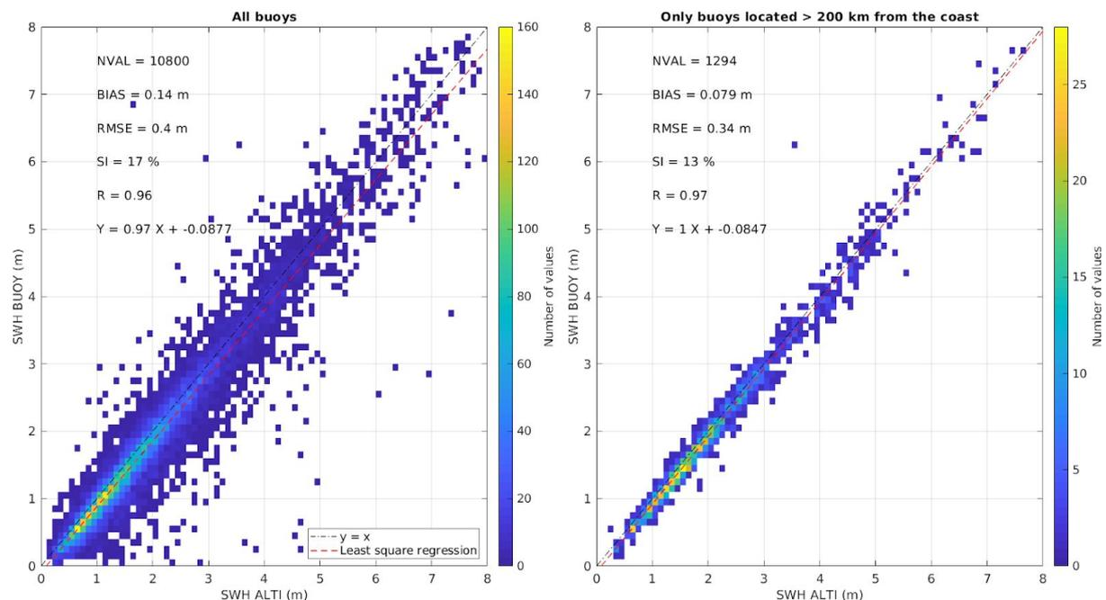
Figure 7. Comparison between Saral and wave buoy swh measurements during year 2014, when all wave buoys are considered (left) and when only wave buoy 200km away from the coast are considered (right).
