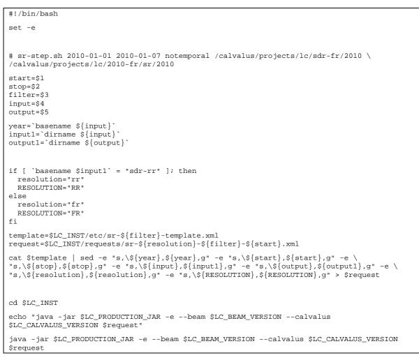
Figure 5-12: Wrapper script example (Sample aggregation processor call) for Calvalus
