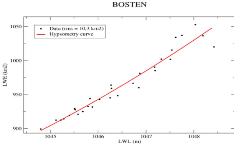
Figure 12: the hypsometry accuracy on Lake Bosten. Red curve represent the theoretical hypsometry determined by least square adjustment of a second order polynomial on the datasets (LWL/LWE). With a 10.3 km<sup>2</sup> of RMSE this represents approximately 1% of total area of the lake.
