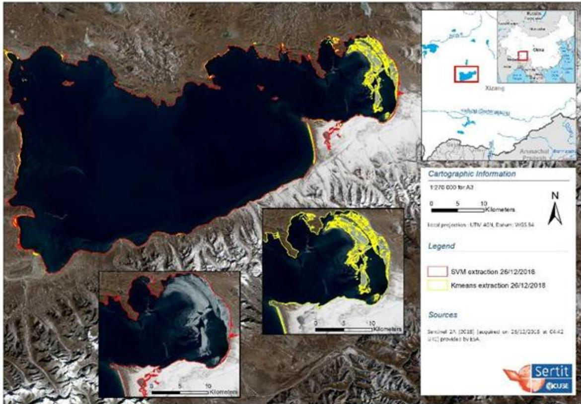
Figure 10: Confusion/commission between Ice and water when exploiting a KMeans approach rather than SVM at Namtso lake (PR China)
