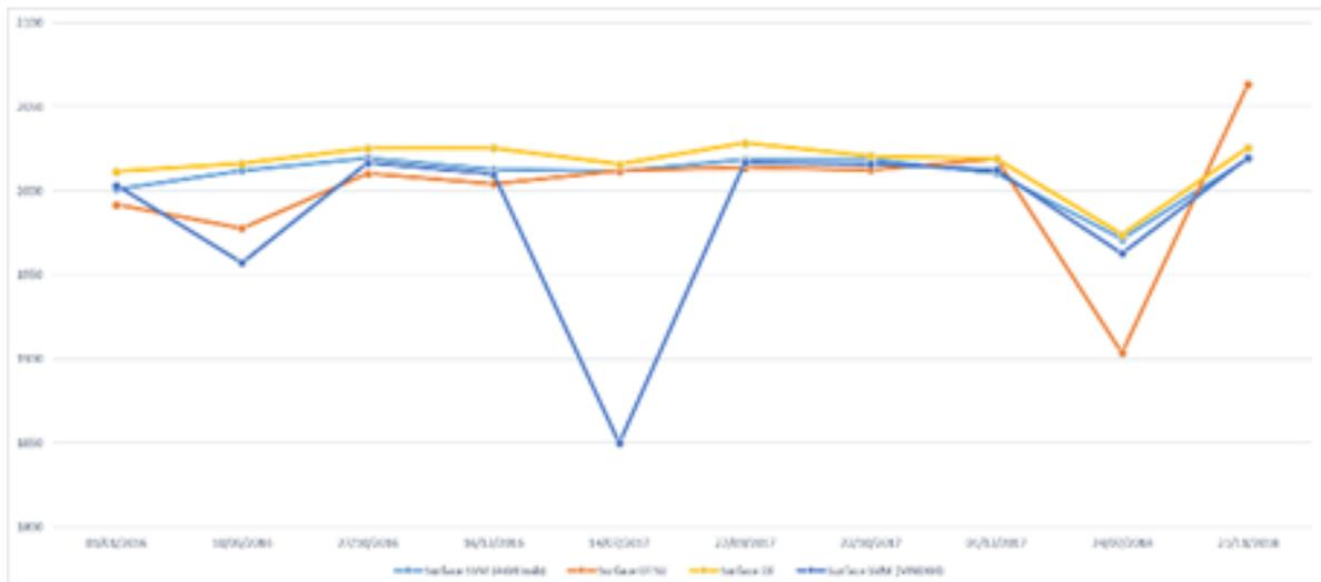
Figure 6. Sensitivity of the MNDWI (dark blue) to sun glint, compared to the AWEI (light blue), yielding a reduced water surface area in case of MNDWI for the sun glint affected scene on 14 July 2017 (low point in time series) shown in Figure 3
