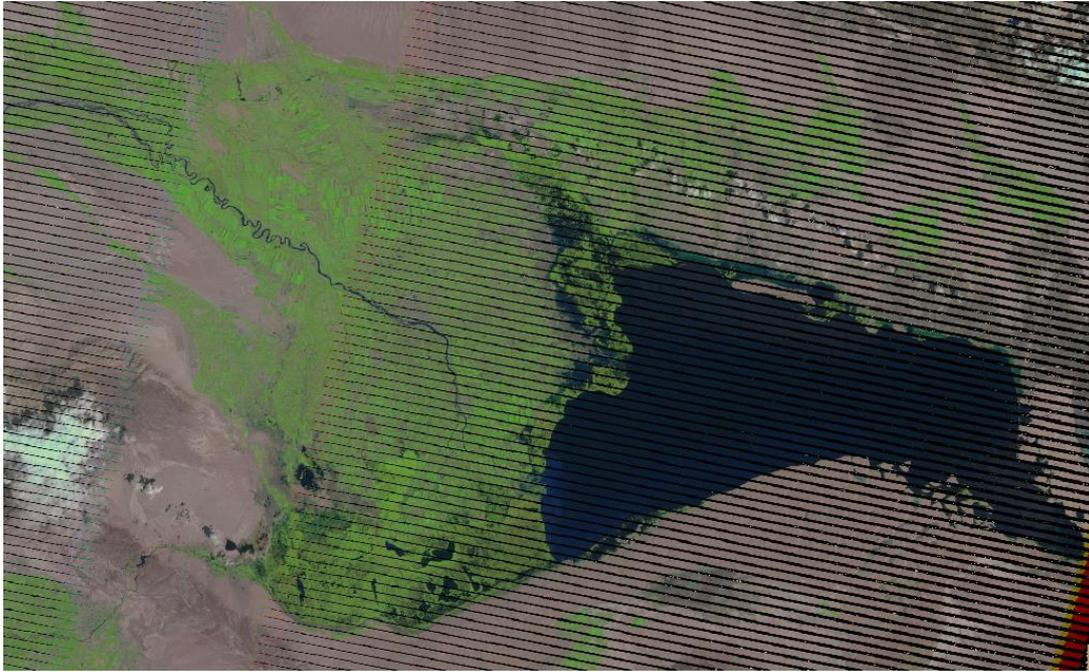
Figure 9: detectors errors on landsat 7 sensors acquired on the 2003-08-09 over Bosten lake
