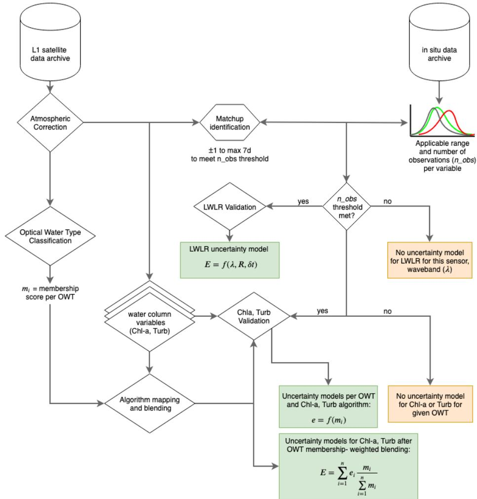
Figure 22 Flow chart of the end-to-end validation of LWLR products against in situ observations, resulting in uncertainty models.
