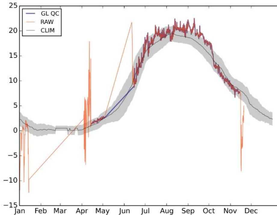
**Figure 8** Illustration of quality control results, in this case for Lake Huron in year 2002. The red line is the received in situ data: when thin, this indicates periods failing quality control, and when thick, data that pass quality control. The black line and grey band show the climatological annual cycle for this location and its inter-annual variability (one sigma).
