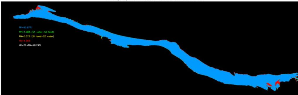
**Figure 3** Comparison between S1 and S2 estimates over Altevattn for 20190927 Blue and red indicates True positives (S1 and S2 both indicate water) and true negatives (S1 and S2 both indicate land). A small fraction of pixels is classified different (yellow and green) by S1 and S2. The overall accuracy is 98%.
