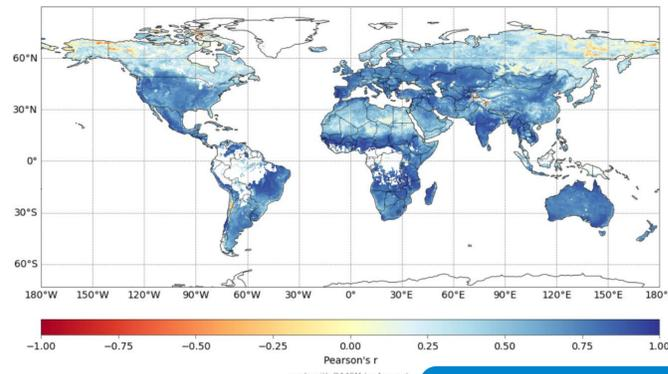
Figure 2: Correlation of the gridded soil moisture COMBINED v06.1 product with the ERA5-Land reanalysis data (created with QA4SM.eu)
