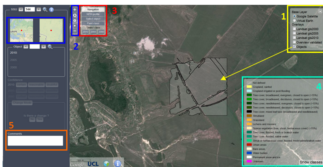
Figure 5. Main page of the validation tool, with the following functionalities: 1) Layer box to display different layouts; 2) Zooming functionalities; 3) Tools box to activate navigation, display NDVI profile, select objects or assign a LC class; 4) Legend description; 5) Comments box to include free text that should help understanding the labelling choices.
