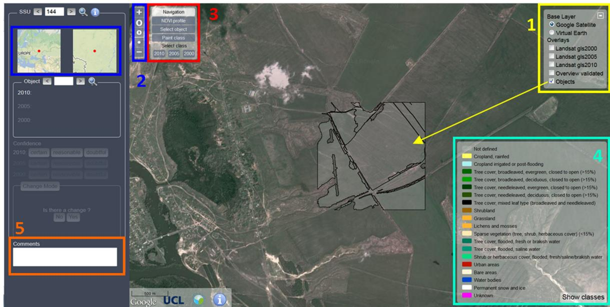
Figure 9. Main page of the validation tool, with the following functionalities: 1) Layer box to display different layouts; 2) Zooming functionalities; 3) Tools box to activate navigation, display NDVI profile, select objects or assign a LC class; 4) Legend description; 5) Comments box to include free text that should help understanding the labelling choices.
