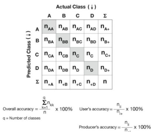
**Figure 3. Layout of a typical confusion or error matrix, showing the computation of user's and producer's accuracies (from [8]). The fields in grey mark the correspondence between classification and labelling by the expert.**
