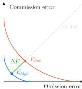
Figure 13. Pareto boundaries for a high and a low spatial resolution in red and blue, respectively. The area below the boundary is a region of unreachable accuracy because of resolution-dependent errors. The resolution error  $E$  corresponds to the intersection between the Pareto boundary and the 1:1 line. The distance between the resolution error for the low and the high resolution is the resolution-dependent error  $\Delta E$  (represented in green) [28].
