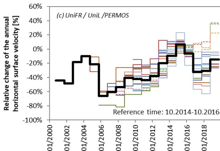
**Figure 5.** Relative evolution of the horizontal surface velocity of rock glaciers in Swiss Alps based on annual terrestrial geodetic surveys. The bold line is the mean ( $n = 1$  to 7 depending on the year).
