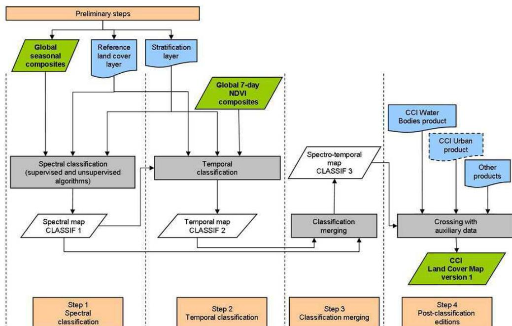
Figure 3-3: LC classification processing chain inherited from prototype
