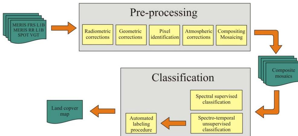
Figure 5-7: Components of the production and development subsystem involved in the LC CCI processing workflow (taken from [RD 3]). A more detailed breakdown is shown in Figure 3-1 and Figure 3-2.
