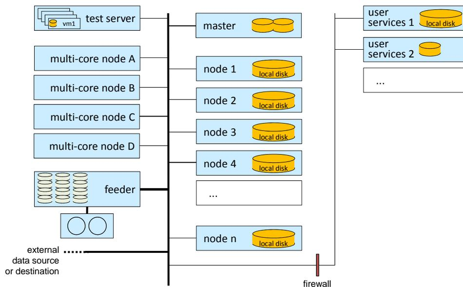
Figure 2-5: LC cluster with two types of nodes for data-intensive pre-processing and for computing-intensive classification
