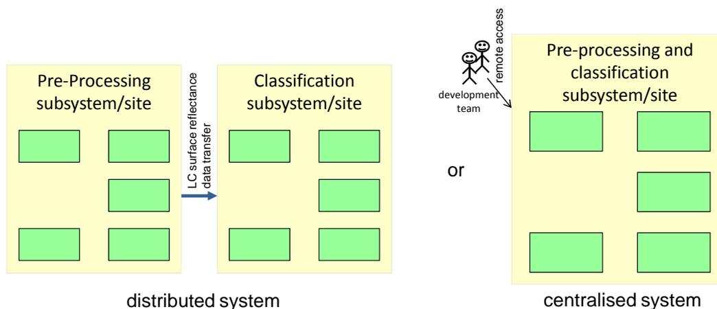
Figure 4-1: Distributed or co-located LC processing infrastructure
