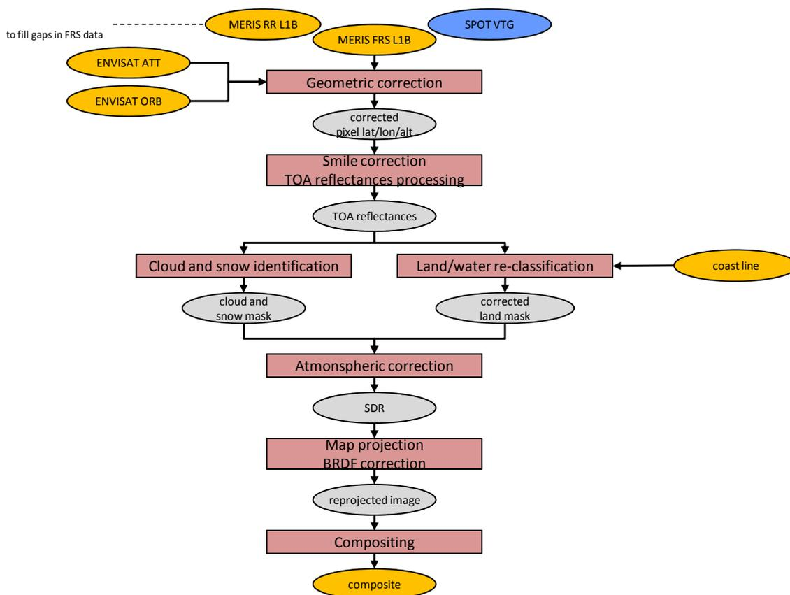
Figure 3-1: LC pre-processing chain inherited from prototype
