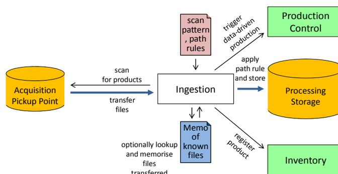
Figure 5-9: Ingestion function to pull input data from a pickup point of a data provider
