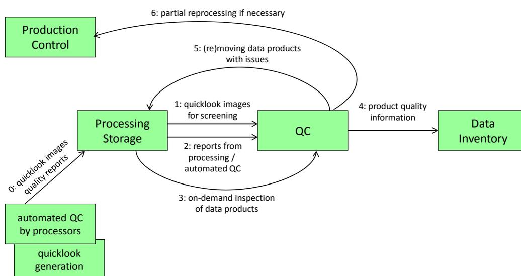
Figure 5-10: Quality check and its interfaces
