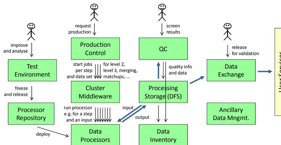
Figure 5-8: Components of the production and development subsystem involved in a workflow for LC CCI processing
