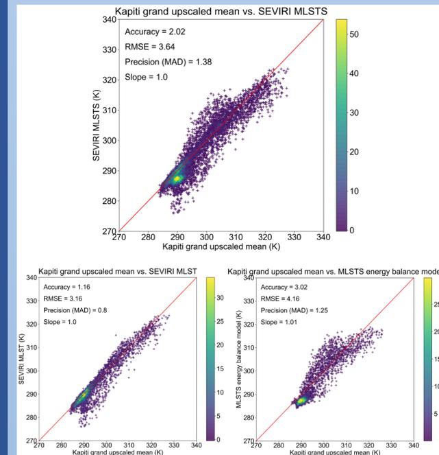
Figure 4. Top: Mean upscaled Kapiti ground LST against the new LSA-SAF all weather product. Bottom left: at times of clear sky, SEVIRI TIR observations. Bottom right: output of the energy balance model alone, at times of cloud. Clear sky and cloud defined by the SEVIRI cloud mask. Performance is generally good.
