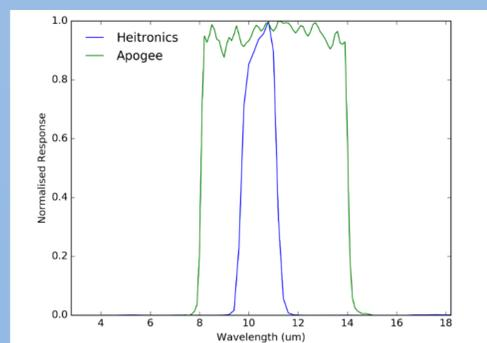
Figure 3. Normalised spectral response functions for a Heitronics KT15.83 IIP radiometer (blue line) and an Apogee SI series radiometer as used by the NASA-JPL radiometers (green line). The Heitronics is considered a narrow-band radiometer whilst the Apogee sits on the border between narrow- and broad-band types.
