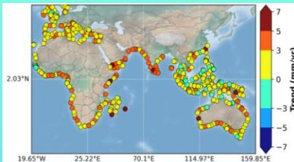
The altimetry-based virtual coastal stations (distance to coast < 6 km) (Colors represent coastal sea level trends in mm/yr over 2002-2020)
