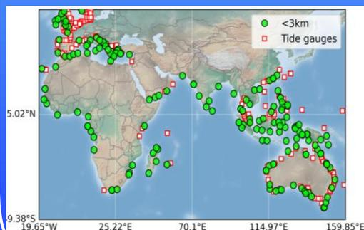
Comparison of altimetry-based coastal sea level with tide gauges records
