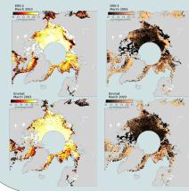
Figure (right): Example of initial ERS-2 pulse deblurring applied on the freeboard. Note the reduction of high values.
