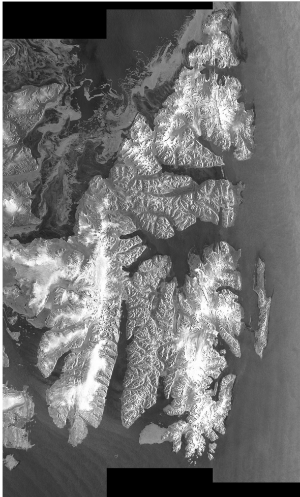
Figure 5: Benchmark image of the averaged backscatter intensity of the S1 image pair 20160210T154421_20160222T154421.pwr. Map is in SAR geometry.
