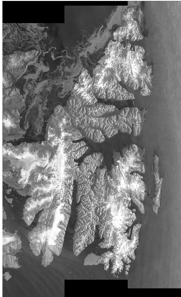
Figure 6: Test image of the averaged backscatter intensity of the S1 image pair 20160210T154421_20160222T154421.pwr. Map is in SAR geometry.
